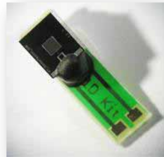
Chip on 3mm x 10mm standard PCB board (including magnets)
