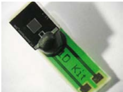
Chip on 3mm x 10mm standard PCB board (including magnets)
